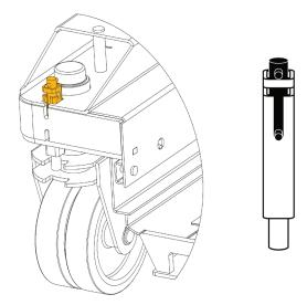
FIGURE 11: Caster Lock Engaged
