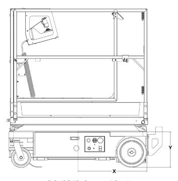
FIGURE 15: Center of Gravity
