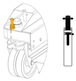
FIGURE 10: Caster Lock Disengaged
