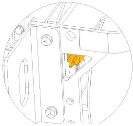
FIGURE 22: Power to Platform Plug
