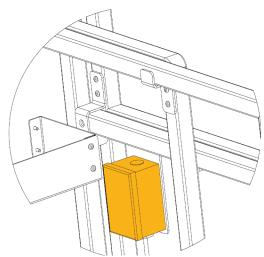
FIGURE 21: Power to Platform Outlet
